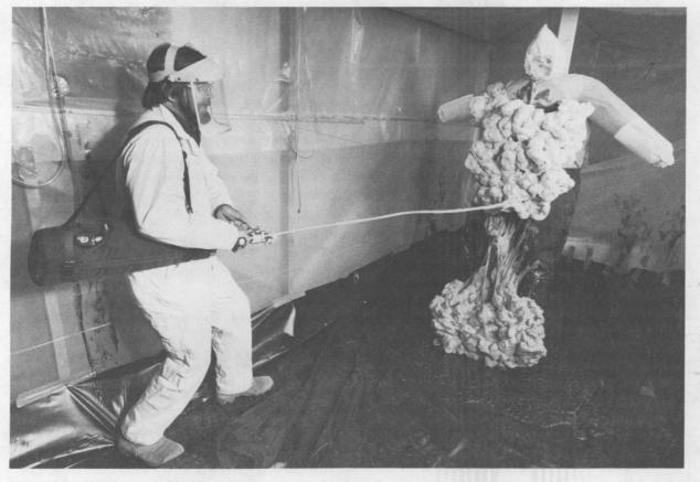
FOAM FOR FELONS — Jeff McDowell of Access Delay Technology Dept. 9611 sprays a mannequin with sticky foam using a new sticky foam gun he built and helped test. The gun is among a relatively new class of "less-than-lethal" weapons for law enforcement that temporarily disable, rather than kill, their human targets. It is likely to get its first use in US prisons. (Photo by Randy Montoya)
